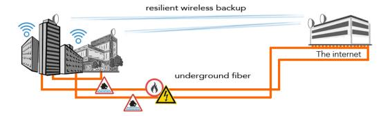
We leverage microwave and millimeter wave for their respective strengths. For instance, microwave wins for distance, but millimeter wave is best for urban environments, where it delivers the highest bandwidth, while also scaling the easiest, because it has the smallest RF (signal) footprint.
